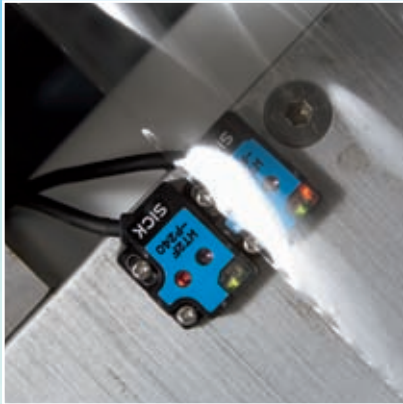
W2 Sensors scan highly transparent films under extreme space restrictions
