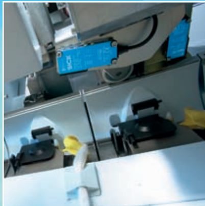
W18 Presence checking in the textile industry
