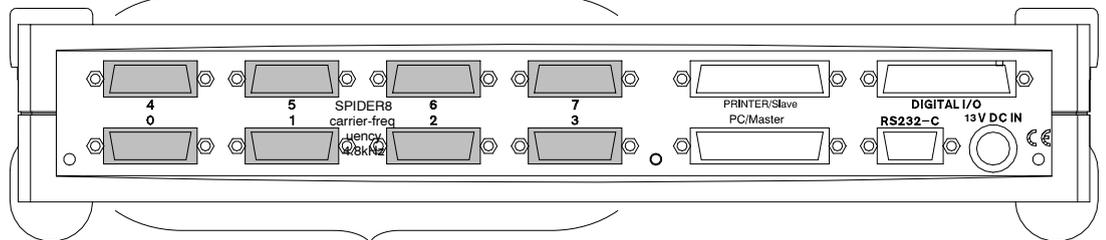
Channel 0 to 3: permanent carrier-frequency amplifier modules
