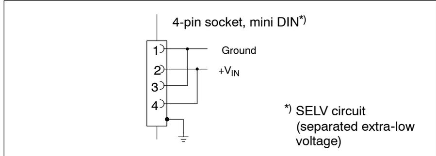
**Fig. B 2:** Pin assignment on 13V DC IN socket
