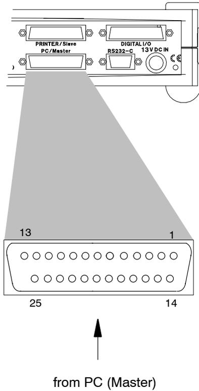
Linking a *Spider8* to a PC or to an upstream *Spider8*.
