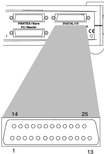
Eight digital inputs and eight I/Os (8-bit input / 8-bit output) are available on this socket besides control signals and status messages. The contacts are not electrically isolated.
