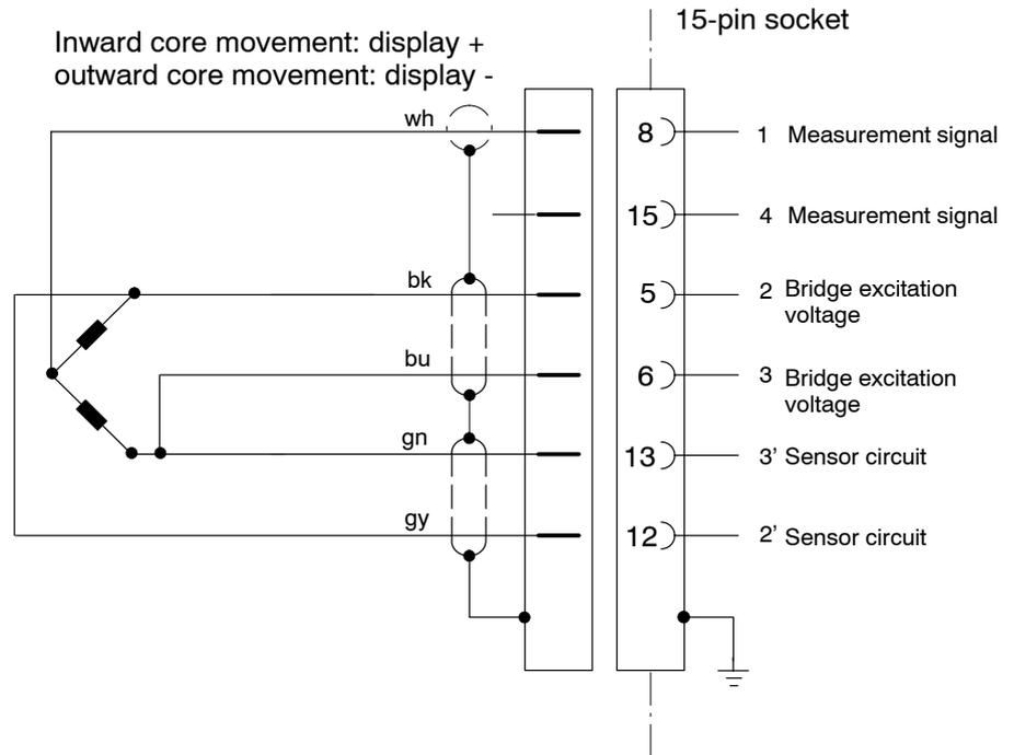
It is not permissible to connect a 3-wire cable that is longer than 3 metres.
