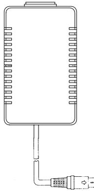
Cable (long) with 4 pins. Mini DIN socket
