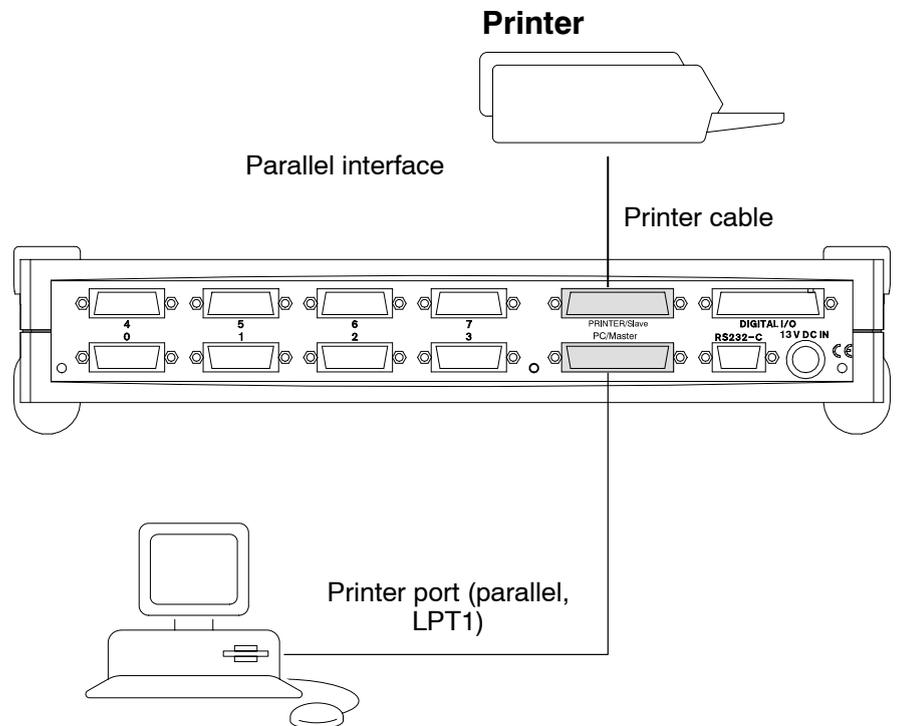
1. Connect the printer cable to the PRINTER/Slave socket (25-pin) on the *Spider8*.
