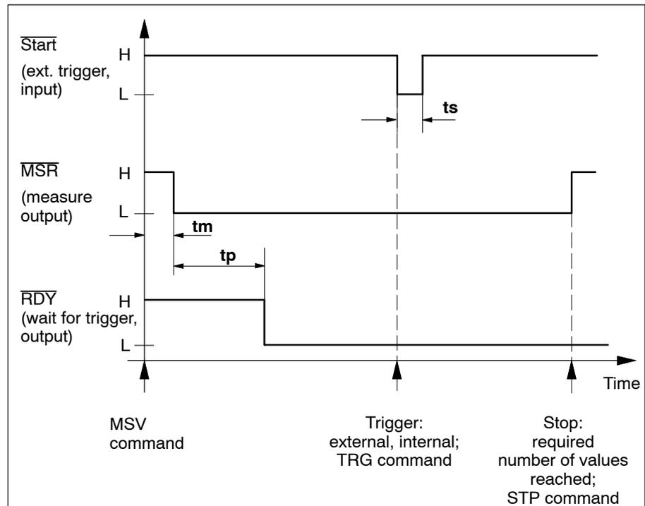
$t_m$  = Synchronisation time (max. 1 set sample time =  $1/\text{sample rate}$ )
