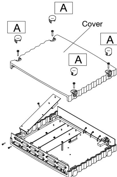
1. Remove the four caps (A) from the top of the *Spider8* housing (prise them up with your thumb).
