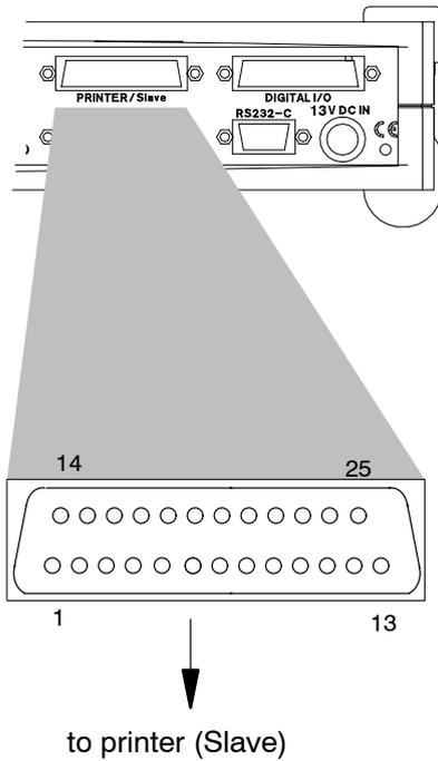
Linking a *Spider8* to a printer or to a downstream *Spider8*.
