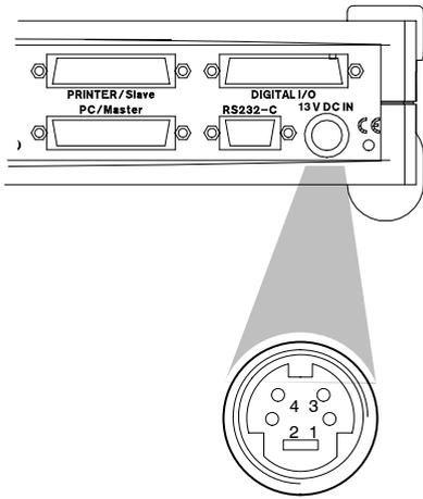
An external power pack (input: 100 - 250VAC; output: 13VDC, 2mA) supplies the DC power to the *Spider8*. The power pack is included in the list of components supplied.
