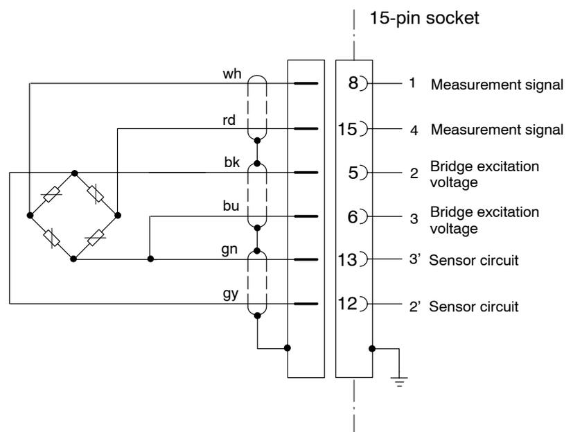
**Connection to carrier-frequency module SR55, SR30**
