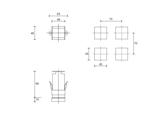
Dimensions: 48x48mm (1/16 DIN) depth 99mm
