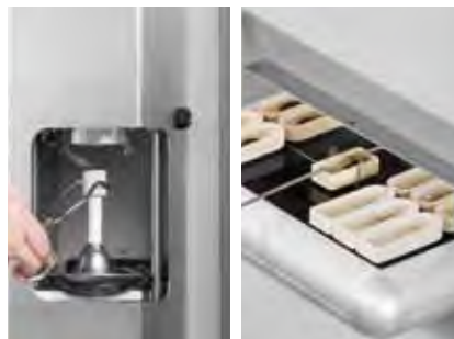
Placing the sample in the induction furnace (left) or the resistance furnace (right)
