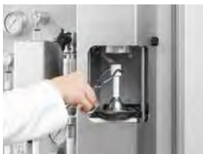
Placing the sample on the pedestal Optional automatic sample loader available
