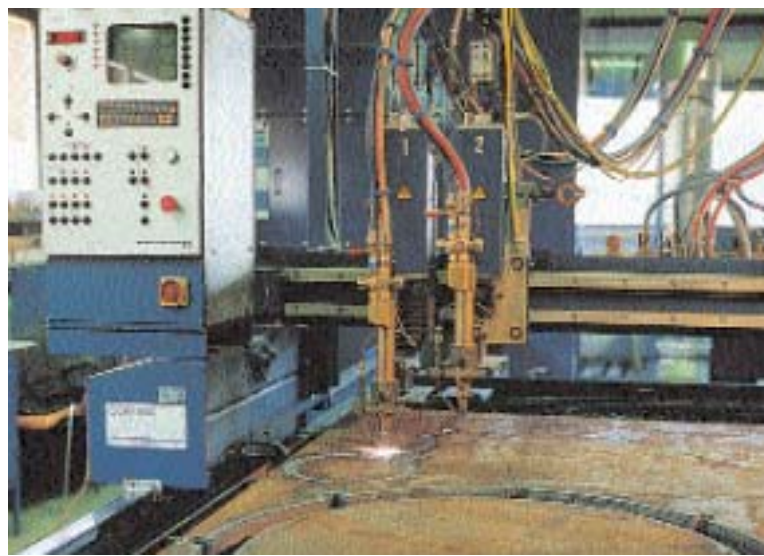
High-value flame-cutting machine for individual components.
